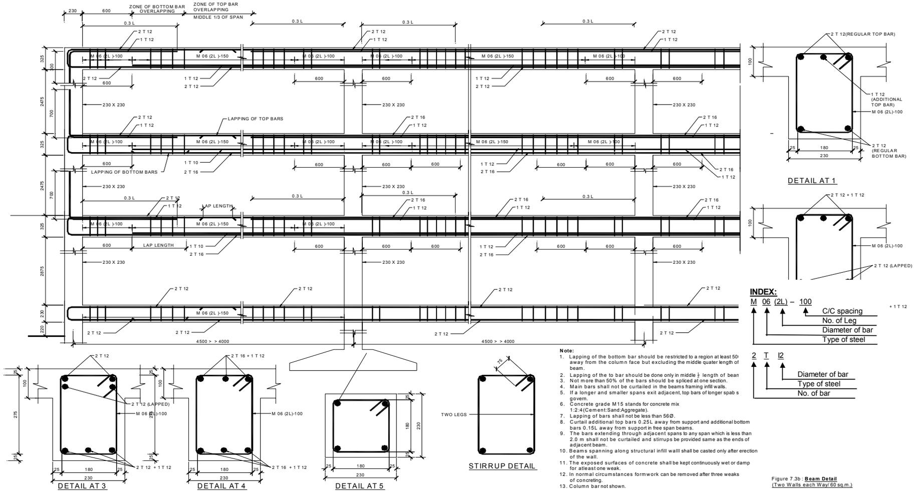
Figure 7.3b : Beam Detail (two walls each way / 60 m<sup>2</sup>)
