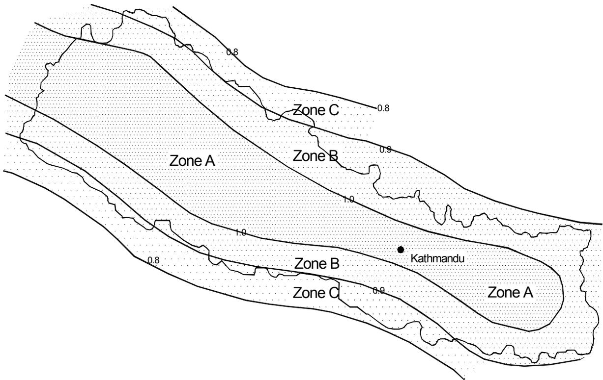
**Figure 1.1 : Seismic Zoning Map of Nepal for this MRT**
