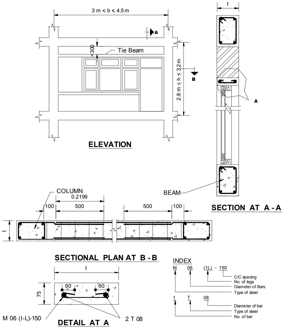
Figure 8.3 : Tie-Band Details for a Non-Structural Wall
