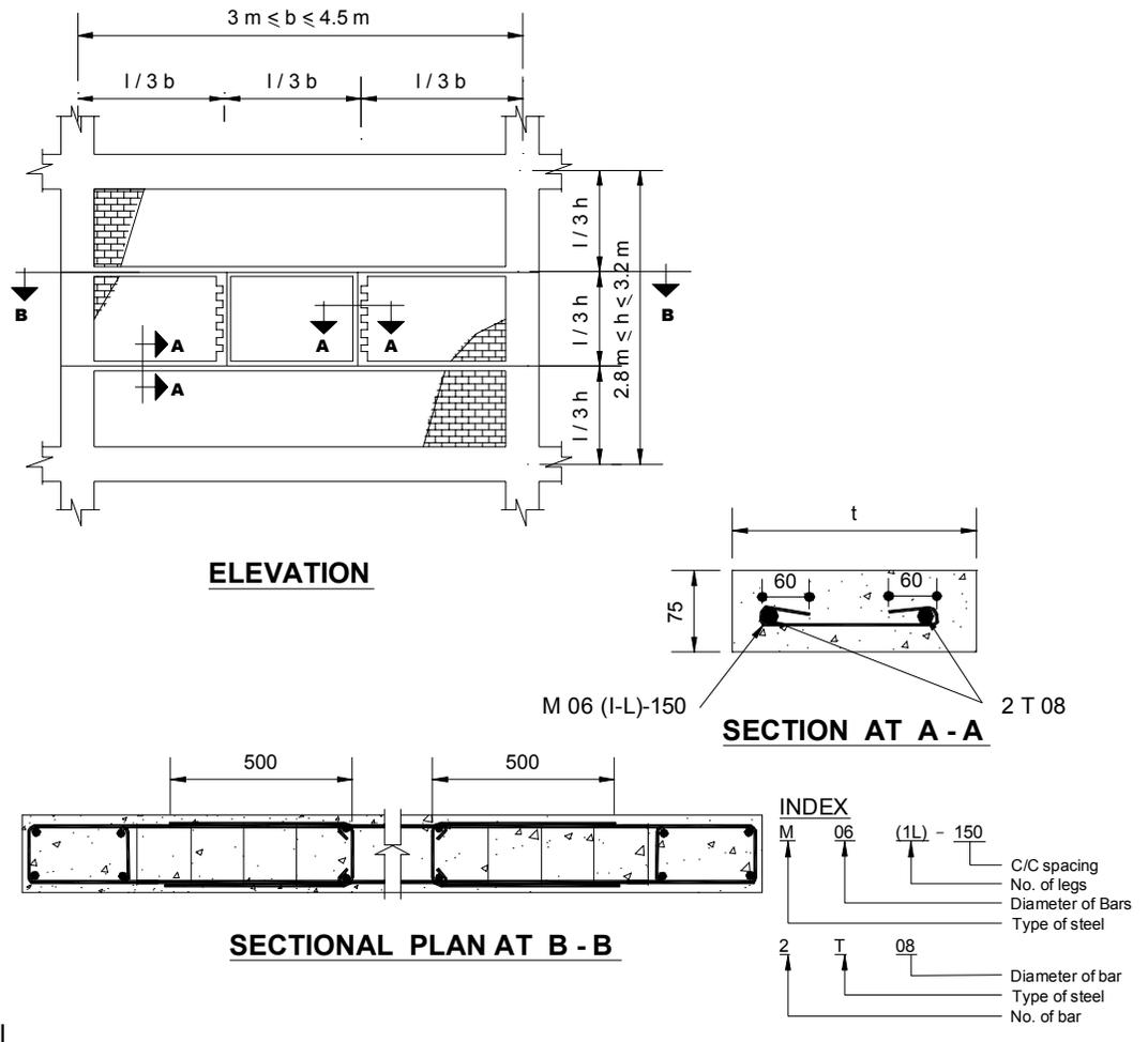
**Figure 8.2 : Details for Opening Stiffening of Infill Wall**
