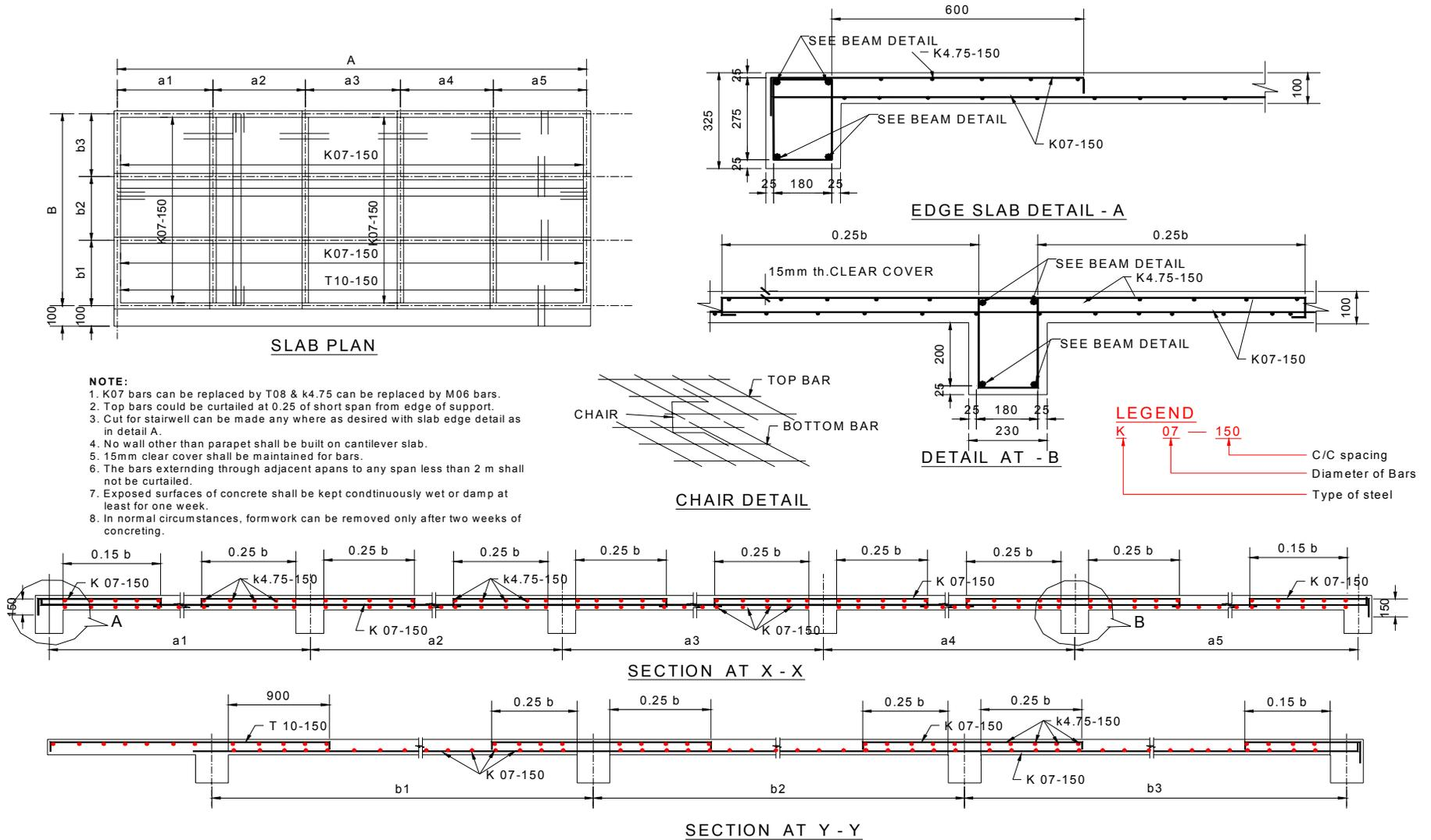
Figure 7.2 : Slab Details
