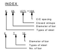
Figure 7.4a : Column Detail (two walls each way / 100 m<sup>2</sup>)
