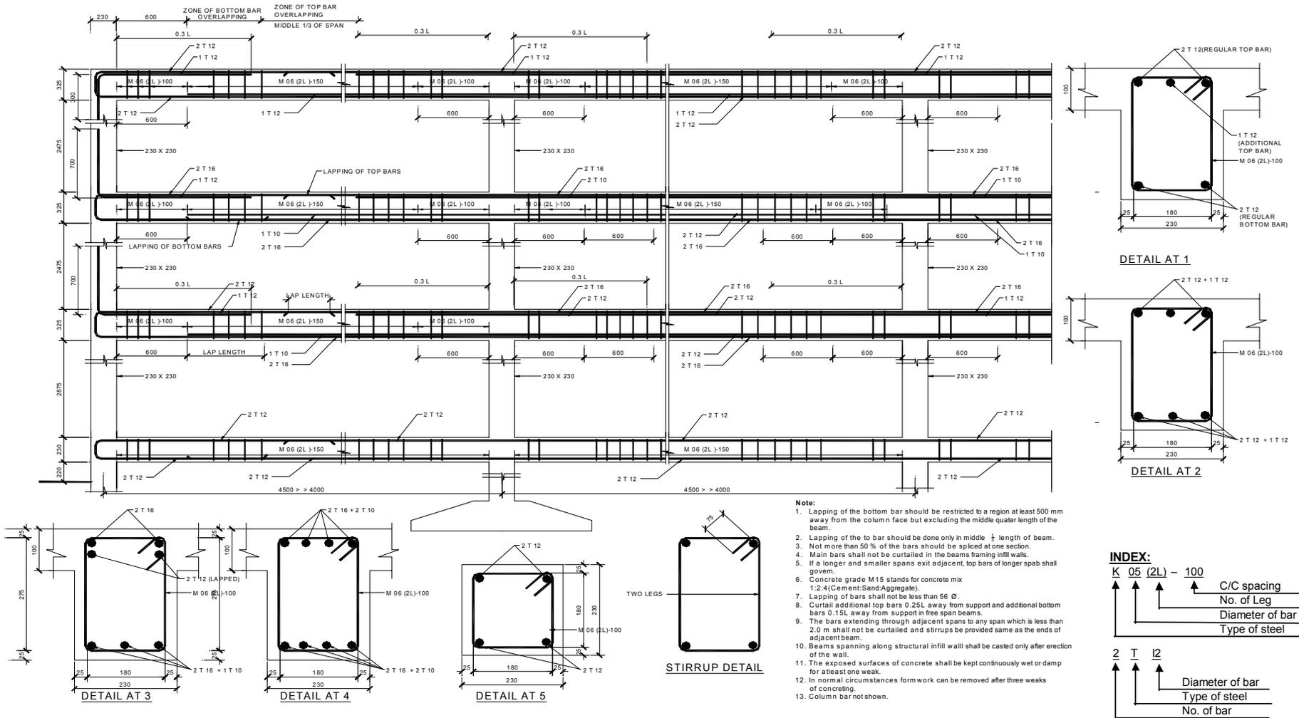
Figure 7.3a : Beam Detail (two walls each way / 100 m<sup>2</sup>)
