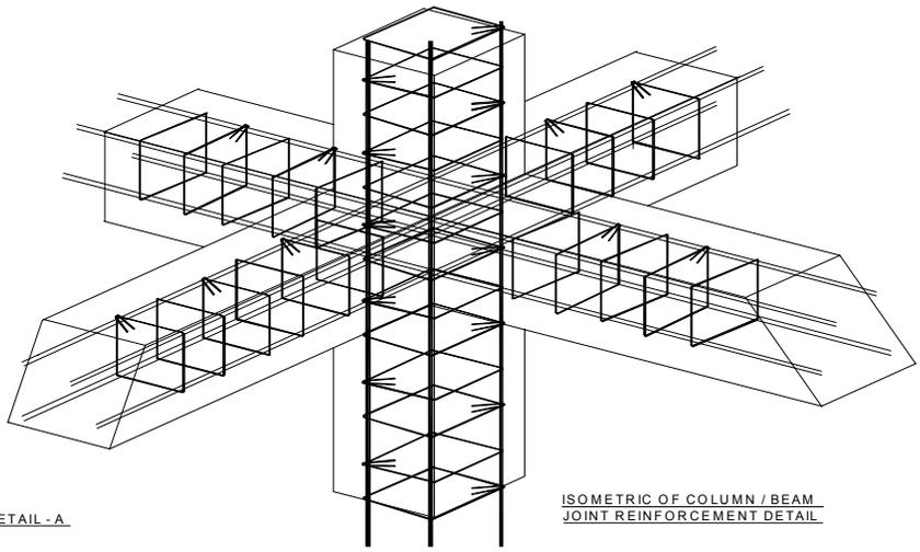
ISOMETRIC OF COLUMN / BEAM JOINT REINFORCEMENT DETAIL
