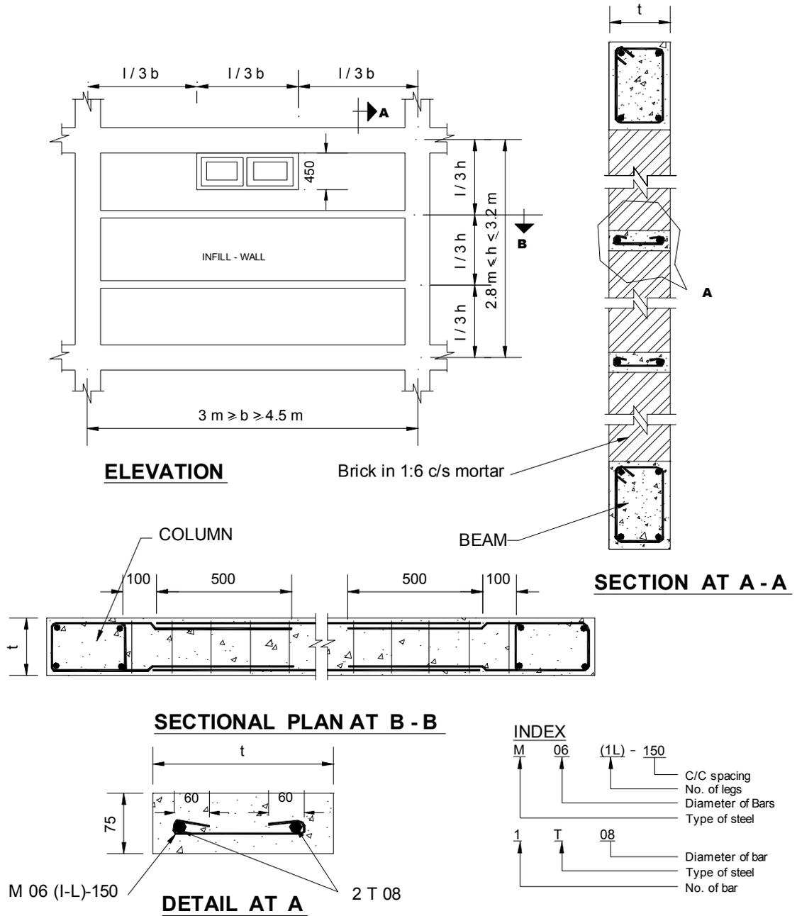
**Figure 8.1 : Tie-Band Detail for Infill (Structural) Walls**
